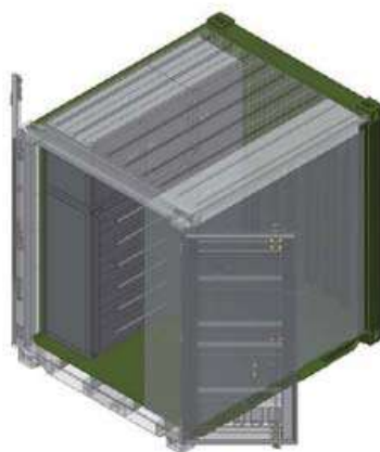
Tricon (Type I) with Modular Cabinet Design Including 24 Total Drawers and 4 Swing-Door Cabinets
