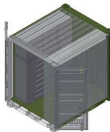
Tricon (Type I) with Modular Cabinet Design Including 36 Total Drawers and 4 Swing- Door Cabinets
