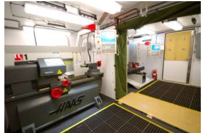
Two Container (20' x 8') Mobile Machine Shop Featuring Mill and Lathe
