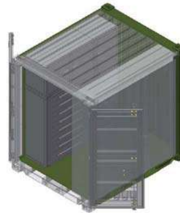
Tricon (Type I) with Modular Cabinet Design Including 36 Total Drawers and 4 Swing-Door Cabinets
