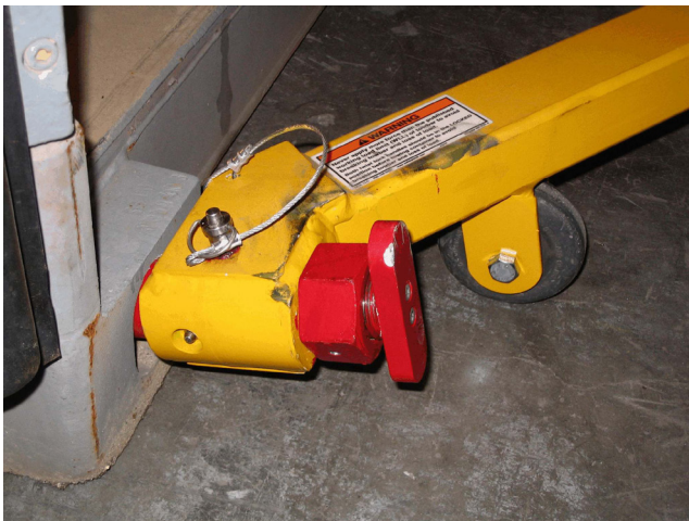
TWISTLOCK ENDS PLUG INTO STANDARD ISO 1161 CORNER FITTING
