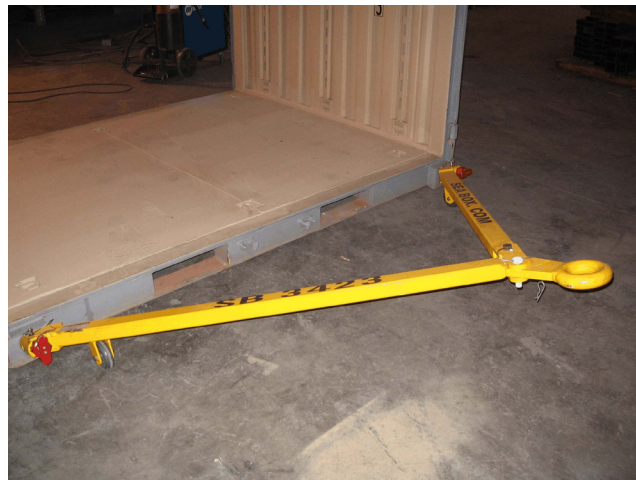
CAPABLE OF TOWING 40' CONTAINERS WEIGHING UP TO 67,200 LBS.
