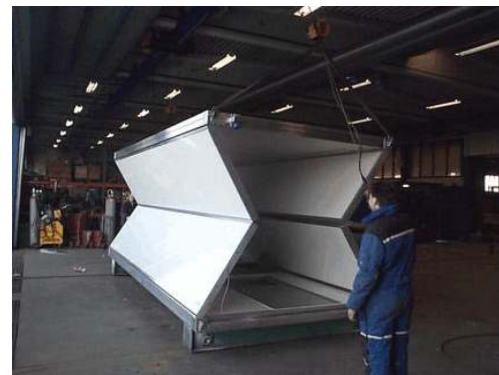
10-minute construction by means of crane or forklift
