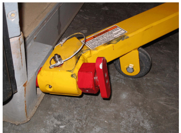
TWISTLOCK ENDS PLUGS INTO STANDARD ISO 1161 CORNER FITTING
