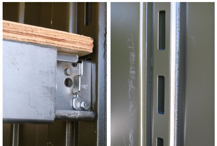
Shoring & Decking Beam engages on vertical "E" track system on ISO Container wall
