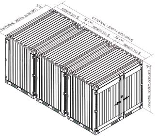
(3) Tricon Containers can be coupled together to form (1) 20' ISO module!
