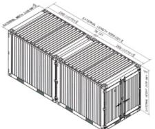
(2) Bicon Containers can be coupled together to form (1) 20' ISO module
