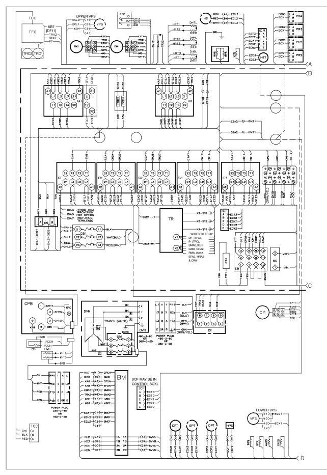
Figure 7-8 UNIT WIRING DIAGRAM - Units with Single Evaporator Fan Capability (Sheet 1 of 2)
