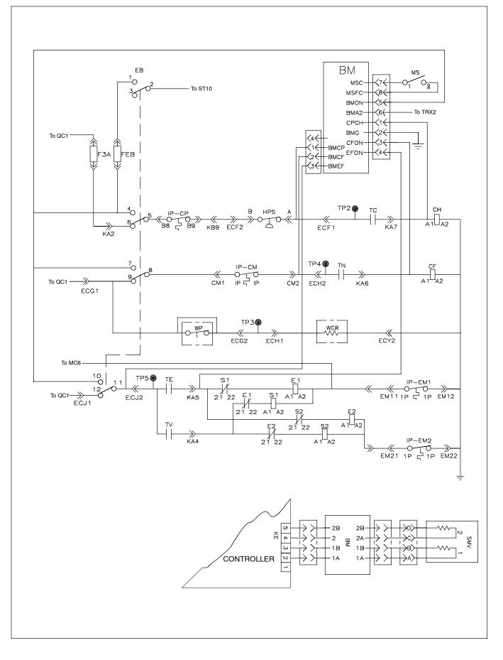
Figure 7-5 SCHEMATIC DIAGRAM - Emergency Bypass
