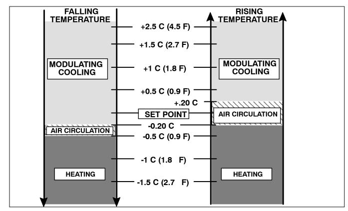
Figure 4-3 Controller Operation - Perishable Mode
