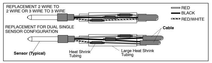
Figure 6-28 Sensor and Cable Splice
