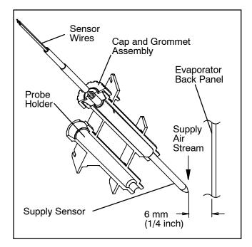
Figure 6-29 Supply Sensor Positioning
