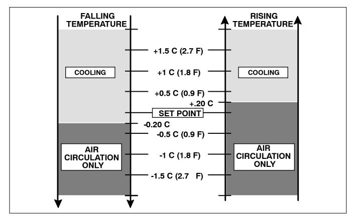
Figure 4-4 Controller Operation - Frozen Mode
