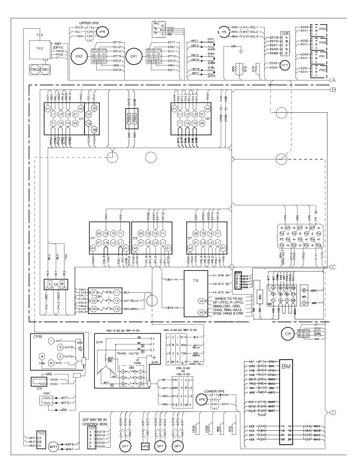
Figure 7-7 UNIT WIRING DIAGRAM - Units with Normal Evaporator Fan Capability (Sheet 1 of 2)
