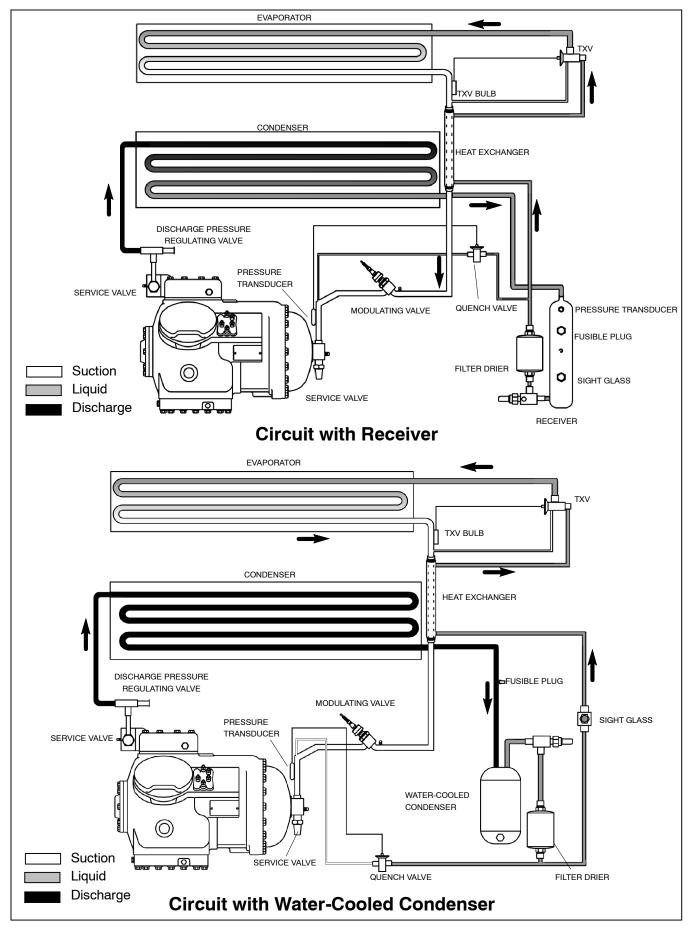
Figure 2-7 Refrigeration Circuit Schematic
