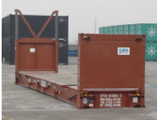
This flatrack operates as a conventional 40ft' Type (4). But within the corner posts there is a high strength telescopic post enabling very tall cargo to be carried, stacked and toplifted by spreader. Full strength is maintained at the maximum height, achieved in five 12in steps.
