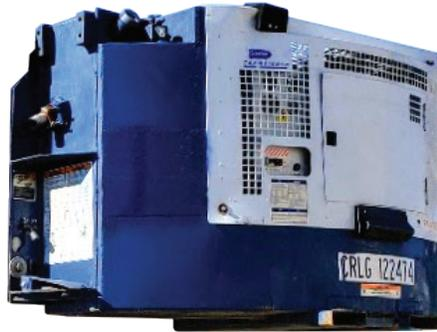
The "Clip On" Generator Set is designed to clip on to the front frame of a refrigerated container. The water cooled diesel generator can provide continuous (single voltage) electrical power to intermodal refrigerated containers. This unit is self contained with an integral fuel tank combined with engine, generator, battery and all operating controls.
